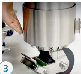
3 Push the 'set-down shims' outward so the height of the column can be adjusted using the pendant and the bottom plate carrier rests on the ground
