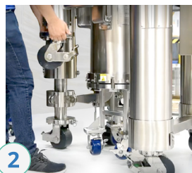
2 Retract the telescoping legs and lock them in place
