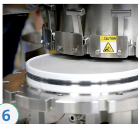
6 Elevate the column to expose the bottom plate resting on the undercarriage, which pivots on a swing-out arm for routine maintenance
