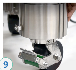
9 Push the set down shims back inward
