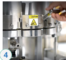
4 Lift the I bars and push to the side to secure in place
