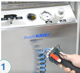
1 Activate the hydraulics and on-board pneumatic pump responsible for raising the column
