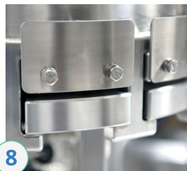
8 Lower the column, pull down the I bars to secure the bottom plate to the column and lift the system once again
