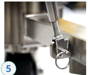
5 Attach the clevis pins and the turn buckles, when necessary
