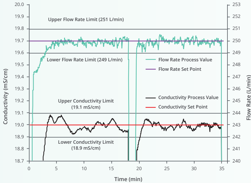
Figure 1. MOTIV holding the conductivity set point of saline solution to within \pm 0.1 mS/cm at a total flow rate of 15,000 L/h. At 18 minutes, a 45-second hold interval was implemented to simulate a process disruption and the system pumps were stopped. After resuming operation, the system came back to the target set point within approximately one minute.
